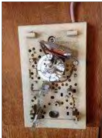
Photo 20 – Liquid mercury is present in thermostats.
