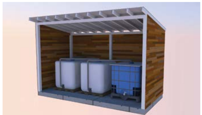
Render of urine collection and sterilization tanks. Image credit: BC Tiny House Collective
